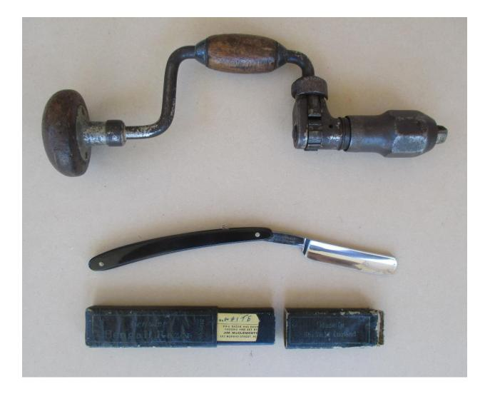
The brace, with drill bit, was in common use for drilling holes. Replaced largely by the hand drill which was easier to use. But now we have electric drills, with rechargeable batteries. How technology changes!
