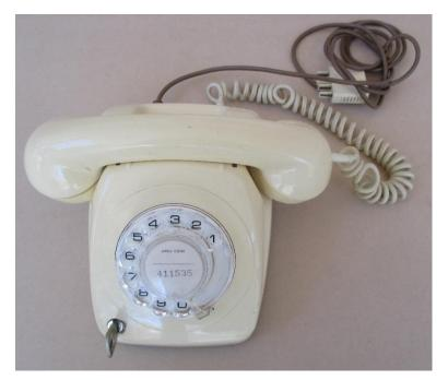
Most of us remember the dial telephone. This one has a key switch on it top prevent illegal use. The dial was replaced by push buttons. And later on, letters were added to the numerals. Then we moved on to handsets which could be used remotely. Now we use mobiles!
