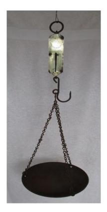
When we buy groceries in a shop we often need to weigh them to determine the price. In days gone by this spring balance was used for weighing. The heavier the weight the longer the spring stretched. All due to gravity! You can still see such scales used today, but they are not very accurate. Try weighing a few things and see which is the heaviest.
